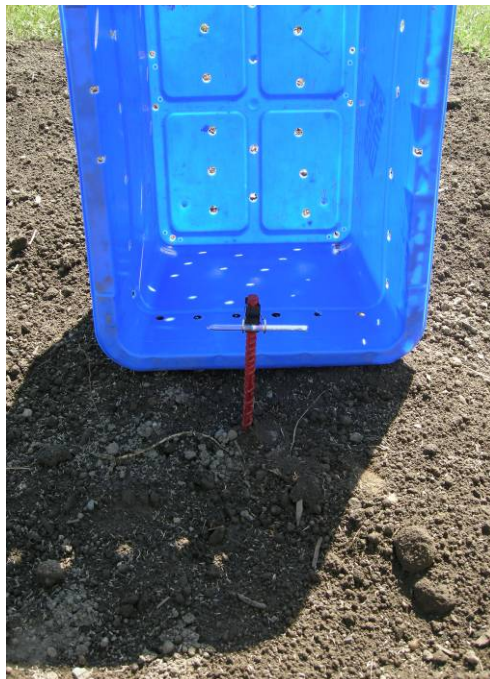
Figure 1. Ammonia loss measurement chamber
